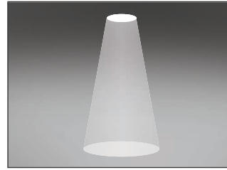
/NB 20° Narrow beam reflector
